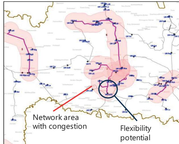
**Figure 4** 110-kV-grid of MITNETZ STROM in Brandenburg with location of flexibility potential
